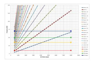
Figure 12 - Campbell diagram with relevant frequencies
