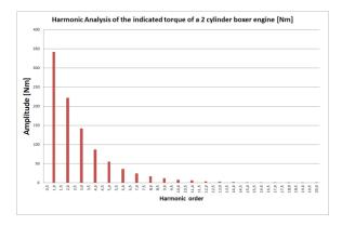
Figure 3 - Harmonic analysis of the indicated torque of a B2 180° crank boxer engine
