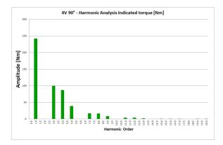
Figure 1 - Harmonic analysis of the indicated torque of a 4V 90° engine
